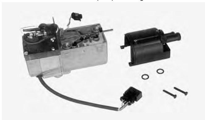
2 Water pump assembly. When mounting, place O-rings on connection on water pump housing
