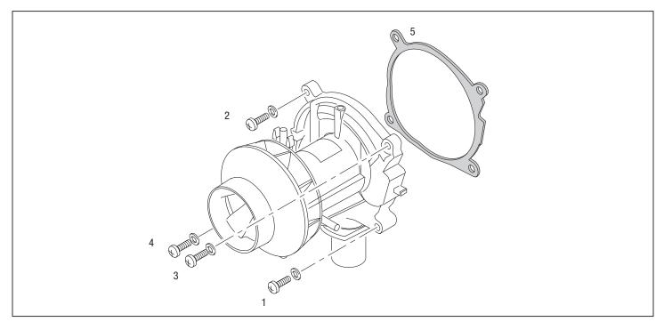
1 - 4 Tighten the fastening screws in this sequence with a tightening torque of 4 <sup>+0.5</sup> Nm (35in•lb)
