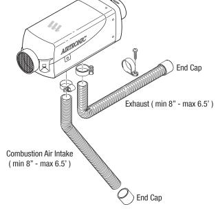
**PLEASE NOTE!** Bends in both the intake and exhaust pipes should be kept to a minimal. For every 90° bend it is recommended to shorten pipe by 16" (40cm).
