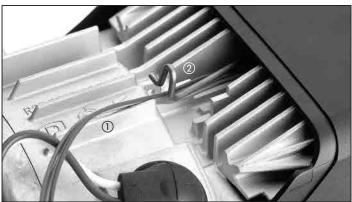
1) Cable harness for overheat/flame sensor clip
