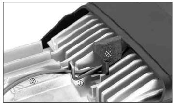
1) Clip 2 Cable harness - overheat/ flame sensor (3) Special tool - only necessary for the AIRTRONIC D2
