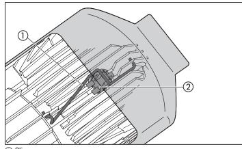
(1) Clip (2) Overheat sensor / flame sensor
