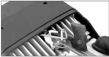
(1) Special tool - only for AIRTRONIC D2 (2) Overheat sensor / flame sensor
