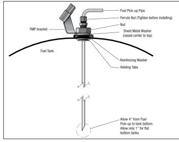
CUSTOM PICK-UP PIPE WITH 1/4" NTP FITTING - OPTION
